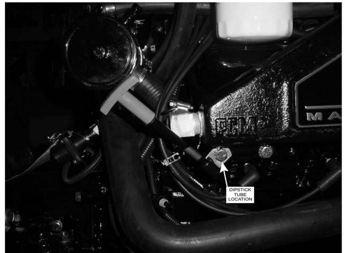
Figure 1-11 FWC V-Drive - Dipstick Tube Relocated
