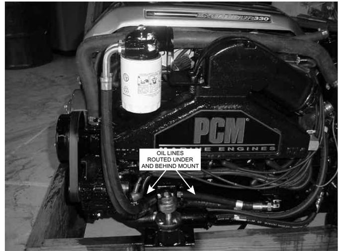
Figure 1-12 Oil Line Routing
