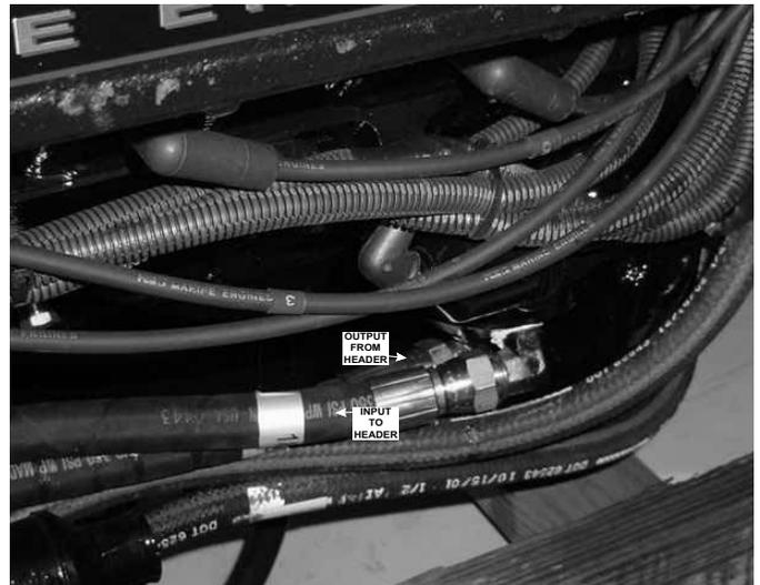
Figure 1-13 Oil Line Connections at Adapter Housing
